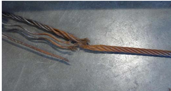
Figure 5 A heavily rusted wire rope.
